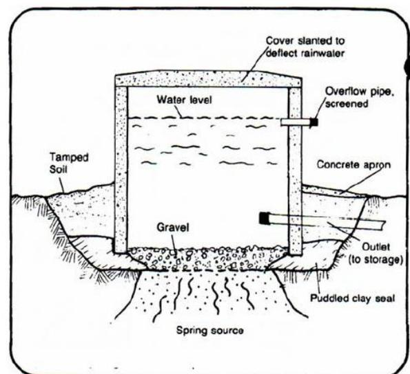
**Figure 3:** Spring box with permeable bottom that will be the model for the improved spring in Parina. (Courtesy of USAID, 1982, available online at [www.lifewater.org](http://www.lifewater.org))
